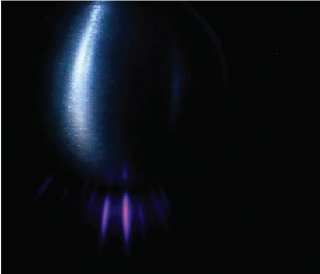
**Figure 1. Direct-current corona discharge of negative polarity on a spherical surface, showing a stage with few moving streamers in blue to purple colours (from Riba et al., 2018, p. 10, fig. 4a left).**
